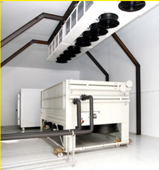
Unit under test in large calorimeter room
